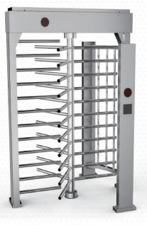
Material Composition: Sus304 Acrylic Size : 1550\*1332\*2230MM Passage Width : 600mm Stock Thickness : 2.0mm+1.2mm Opening Speed : 1~2s Input Signal : switch Quantity (No) Rs485 Total Power : 30 - 60w Operating Temperature Range : -20~70°C Can Be Used Indoors Or Outdoors
