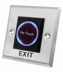
Dimensions:86L\*86W\*16H(mm) Power Supply:DC12-24V Output Contact:NO/NC/COM Material:Stainless steel Operating humidity:0-95% (RH) Mechanical Life: 500,000 Tested aging test qualified Door Type: Hollow door frame installation LED Indicator: Standby blue, Response green Product Weight: 0.11KG Package Quantity: 1 PCS/box, 100 PCS/case Sensitive Distance:5~15cm(Adjustable)
